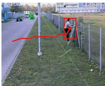
As the person crosses the trip wire next to the fence, the alarm is raised
